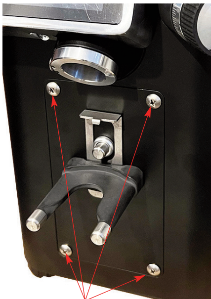
Unscrew the 4 screws of the module
